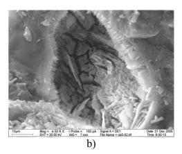
Fig. 1. Microstructure of cement stone and new formations in pore volume of paving blocks after 5 years of service:
